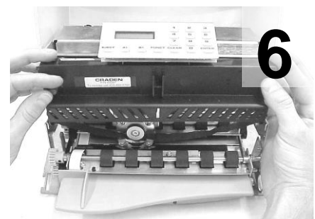
Rotate cartridge into place and snap in. Rotate cartridge drive gear clockwise to align and take up ribbon slack. Push shield up. Lower carriage into operating position. Close cabinet.
